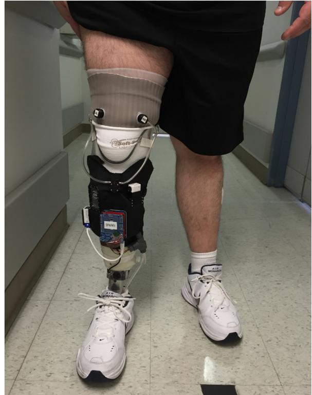
**FIGURE 7-35:** Dynamic Air Exchange prosthesis with black system harness worn by a subject while standing. (Figure used with permission from the authors).
