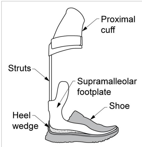
**FIGURE 1:** IDEO–heel wedge–shoe system. The new style heel wedge, shown in hash mark fill, sits in the shoe under the IDEO. (Figure 1 from Ikeda, Ferguson, and Wilken (2017) used with permission from the authors)
