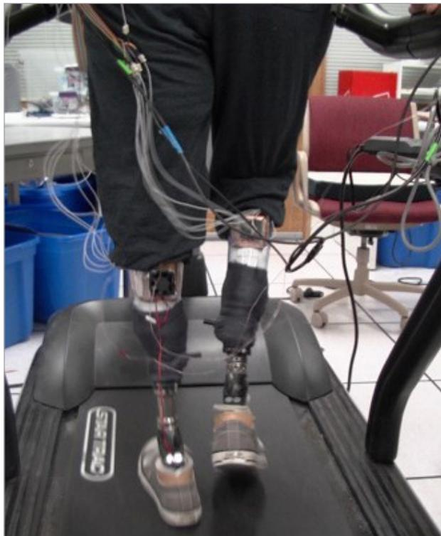
**FIGURE 2:** Bilateral Amputee during Walking Test (Figure used with permission from the authors)
