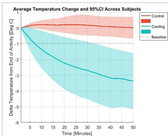
**FIGURE 1:** Average Temperature Change of Five Subjects with and without cooling for 50 minutes after walking (Figure used with permission from the authors)
