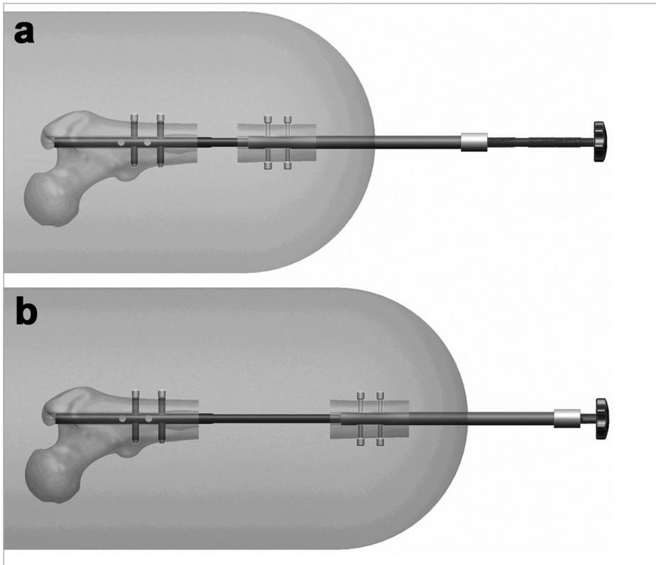
**FIGURE 1:** Schematic of lengthening of residual limb using lengthening device. (Figure from Kuiken et al. (2017) used with permission from the authors)
