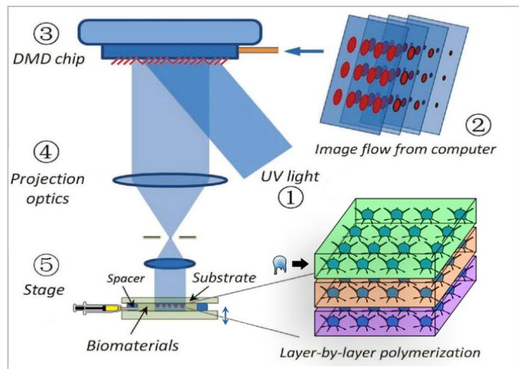
**FIGURE 1:** Schematic diagram of a layer-by-layer bioprinting method with different cells encapsulated in different layers (Figure used with permission from the authors)
